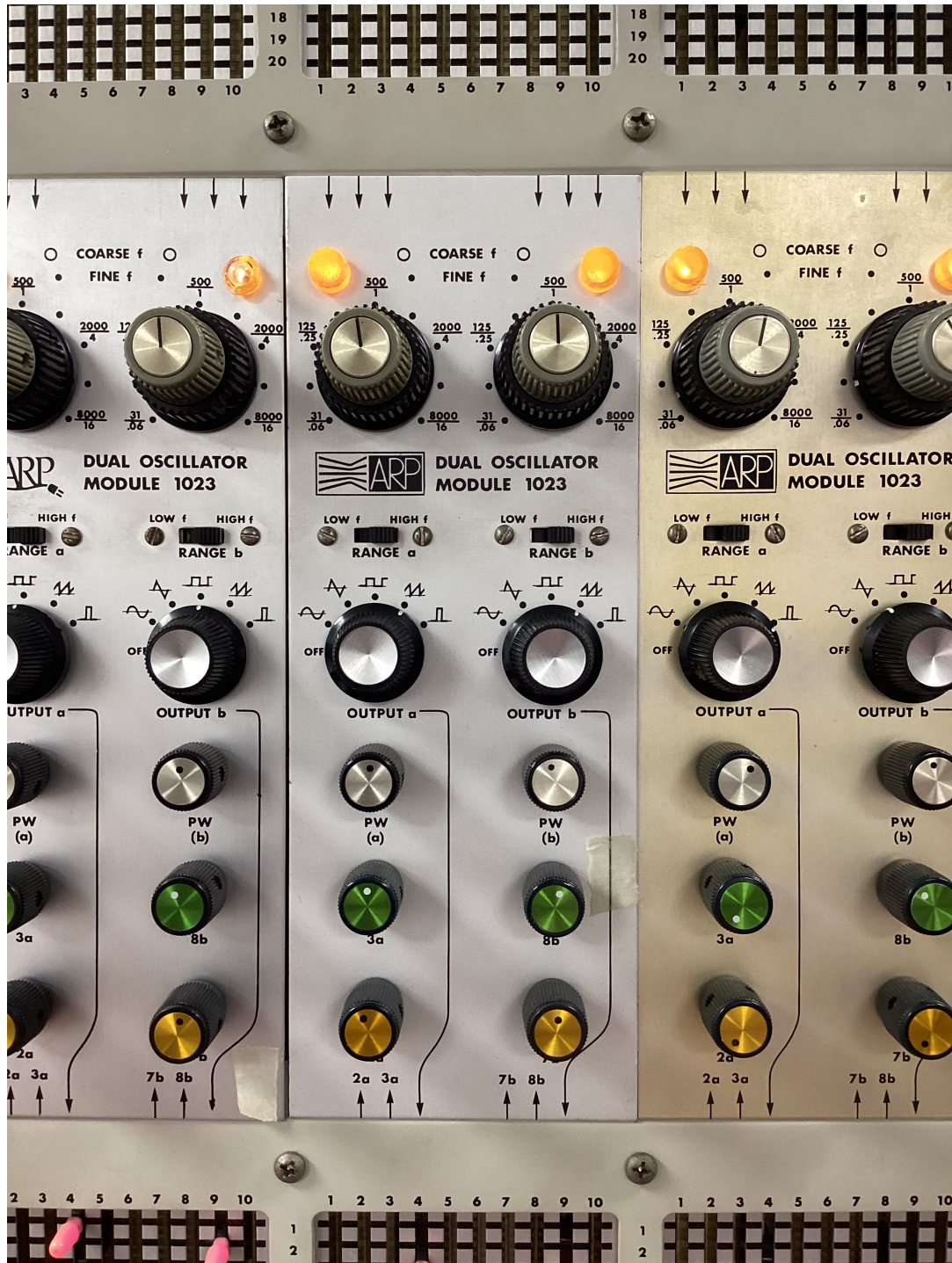
The dual Oscillator boosts fine tune and Coarse tuning, Low and high range, a selection of Wave shapes and PMW Modulation ins and FM in (3a)
